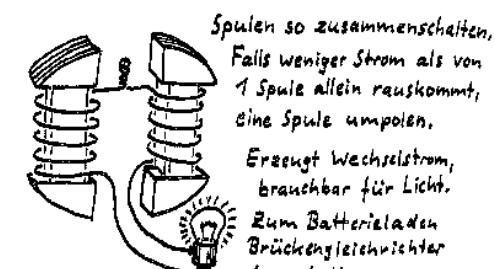
Wire the two coils together. If less current is generated than with a single coil, change the polarity of one of the coils. Generates alternating current, suitable for lamp. Add a bridge rectifier for battery charging.
